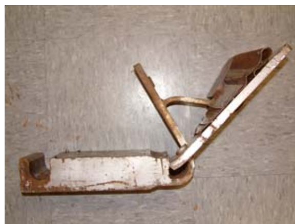
(b) Top plate bent before broken off
