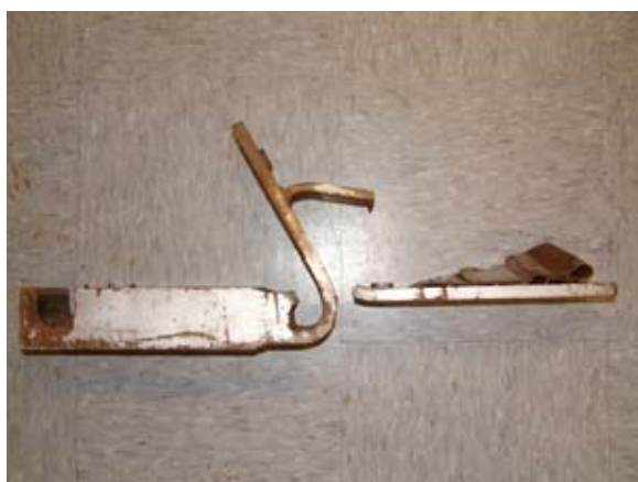
(a) Top plate broken off from head assembly
