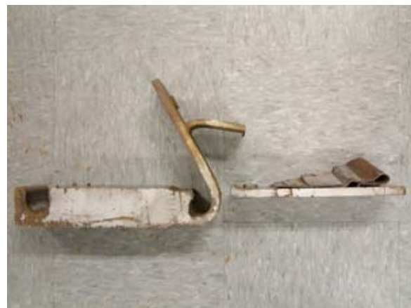
(b) incident towbar head assembly (plate on RHS came off near the top welding position)
