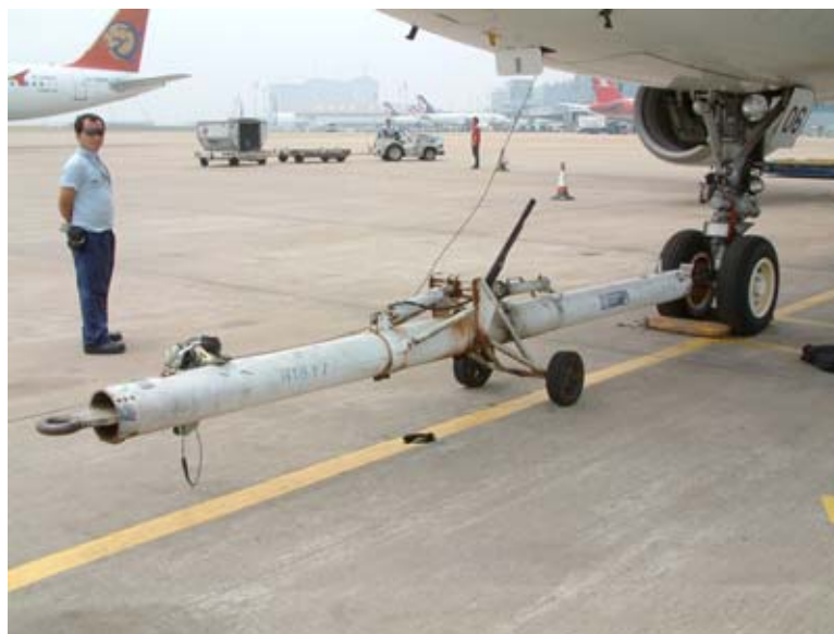
Figure 3-3 : A towbar attaching to the nose undercarriage of an A321 aircraft
