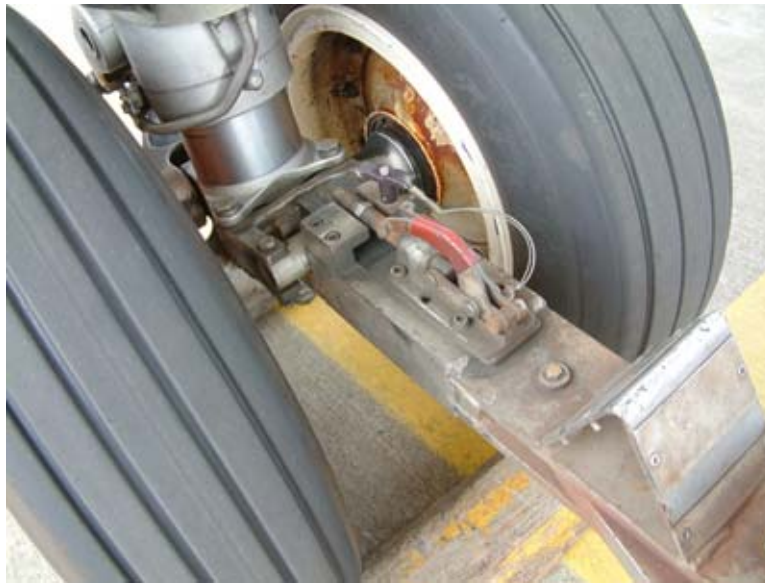
Figure 3-4 : Details of nose undercarriage to towbar head assembly attachment
