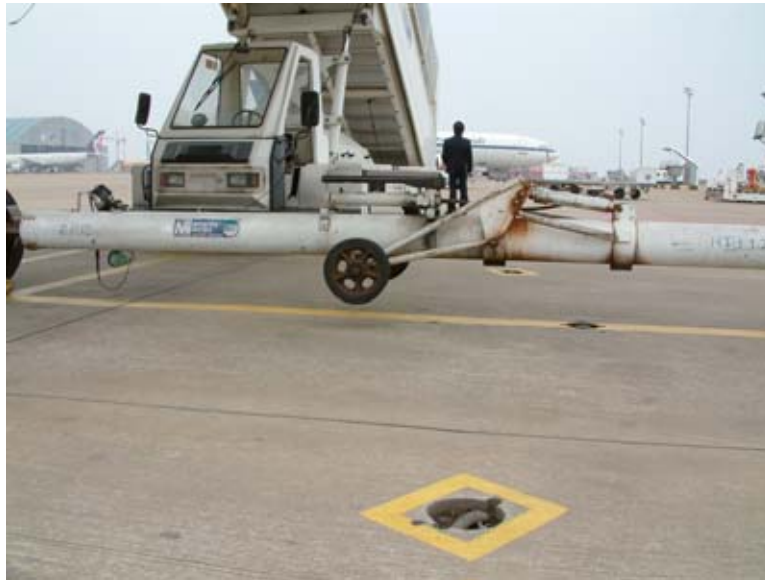
Figure 3-6 : The wheels on towbar were retracted up after attaching towbar to tractor
