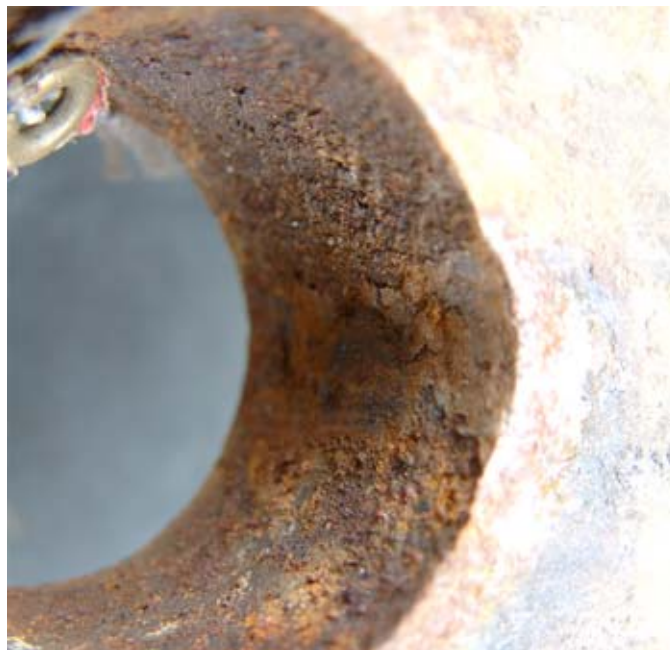
Figure 4-4 : RHS of hole wall dented near top surface
