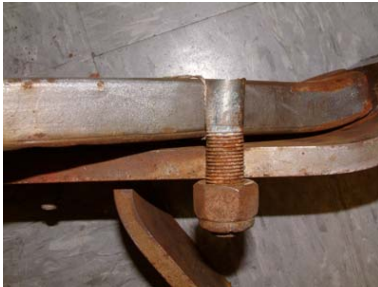
Figure 4-15 : Lower part of the broken bolt (about 16 mm dia.) illustrating fracture between top plate and head-to-tube connector
