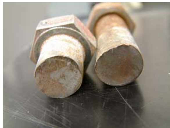
(b) Fracture surfaces of broken bolt
