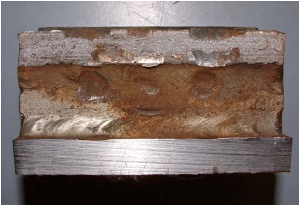
Figure 4-11 : Fracture surface of top plate at head assembly end
