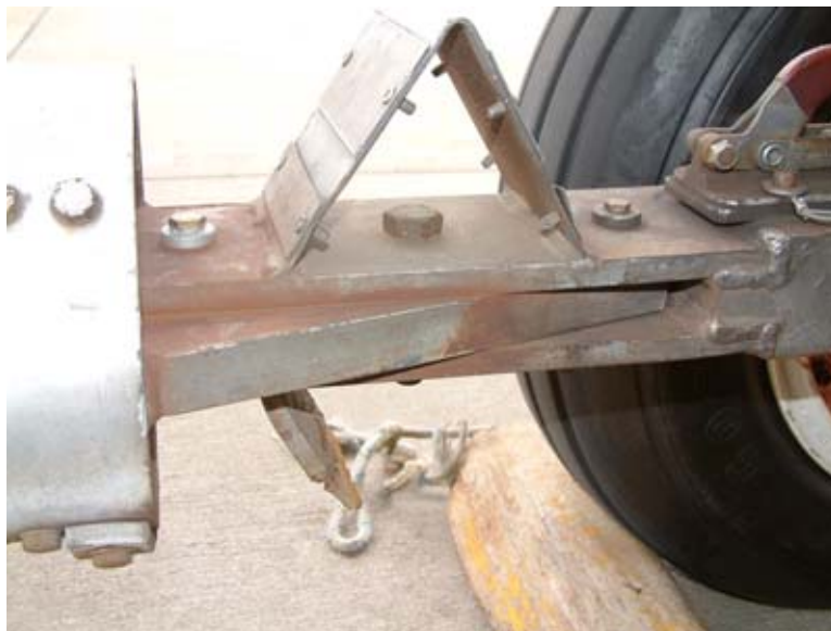
Figure 3-5 : The wheels on towbar were retracted up after attaching towbar to tractor
