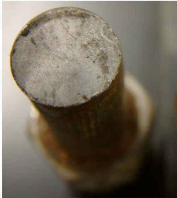
Figure 4-17 : Fracture surface of large shear bolt
