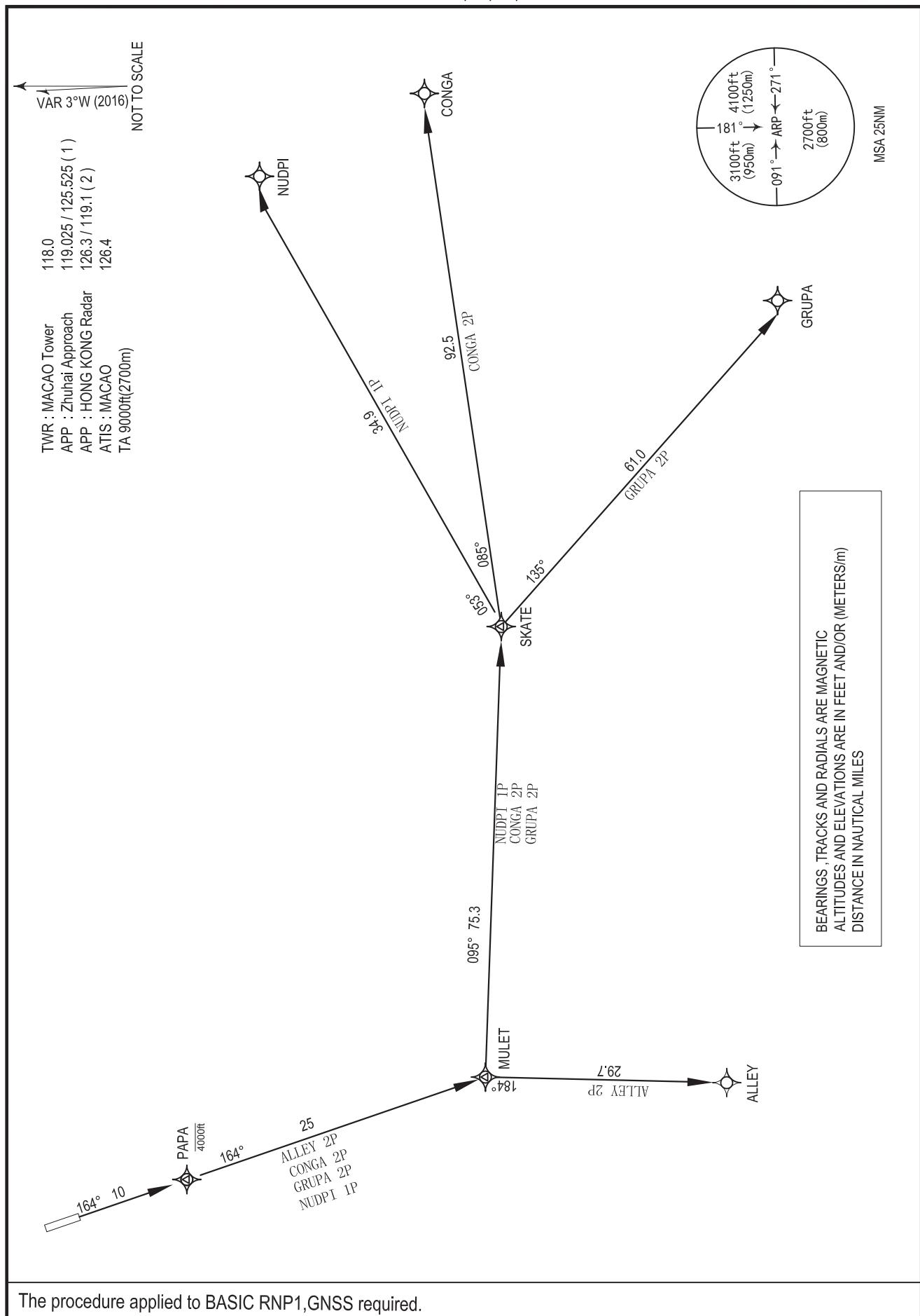
The procedure applied to BASIC RNP1,GNSS required.
