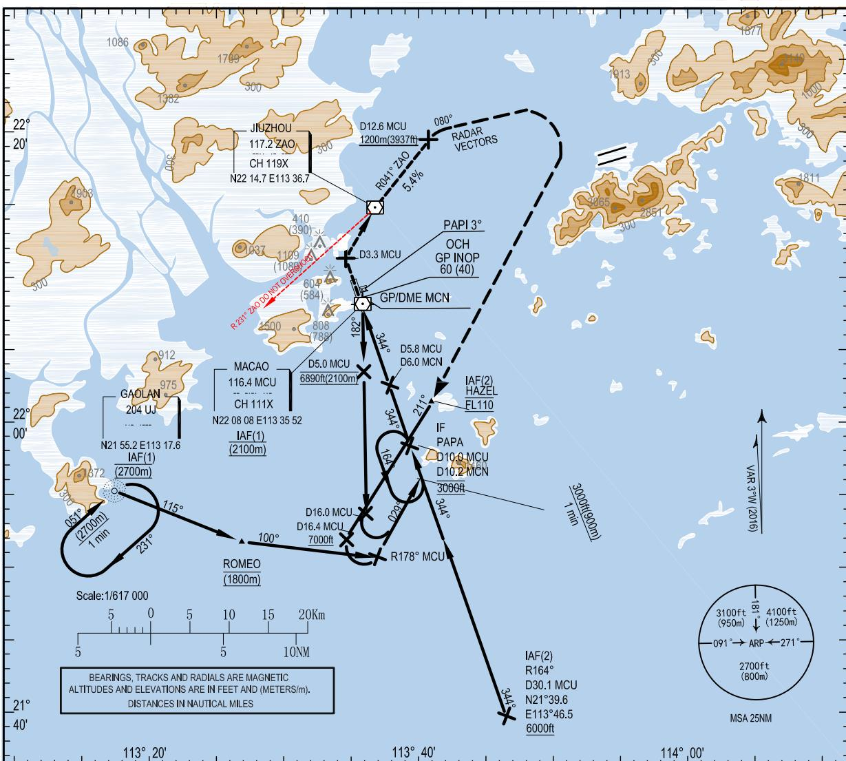
MISSED APPROACH(2);(MN climb gradient 5.4% required until passing 5500 ft) Climb on runway heading to 600 ft (183m). At or before MCU 3.3NM turn right (MAX IAS 185kt) to ZAO, leave ZAO on ZAO R041°. Cross MCU 12.6 NM at or above 1200m (3937 ft) and turn right to track 080°M, continue climbing to 6000 ft (1829 m). Expect radar vectors by Hong Kong ATC to HAZEL.
