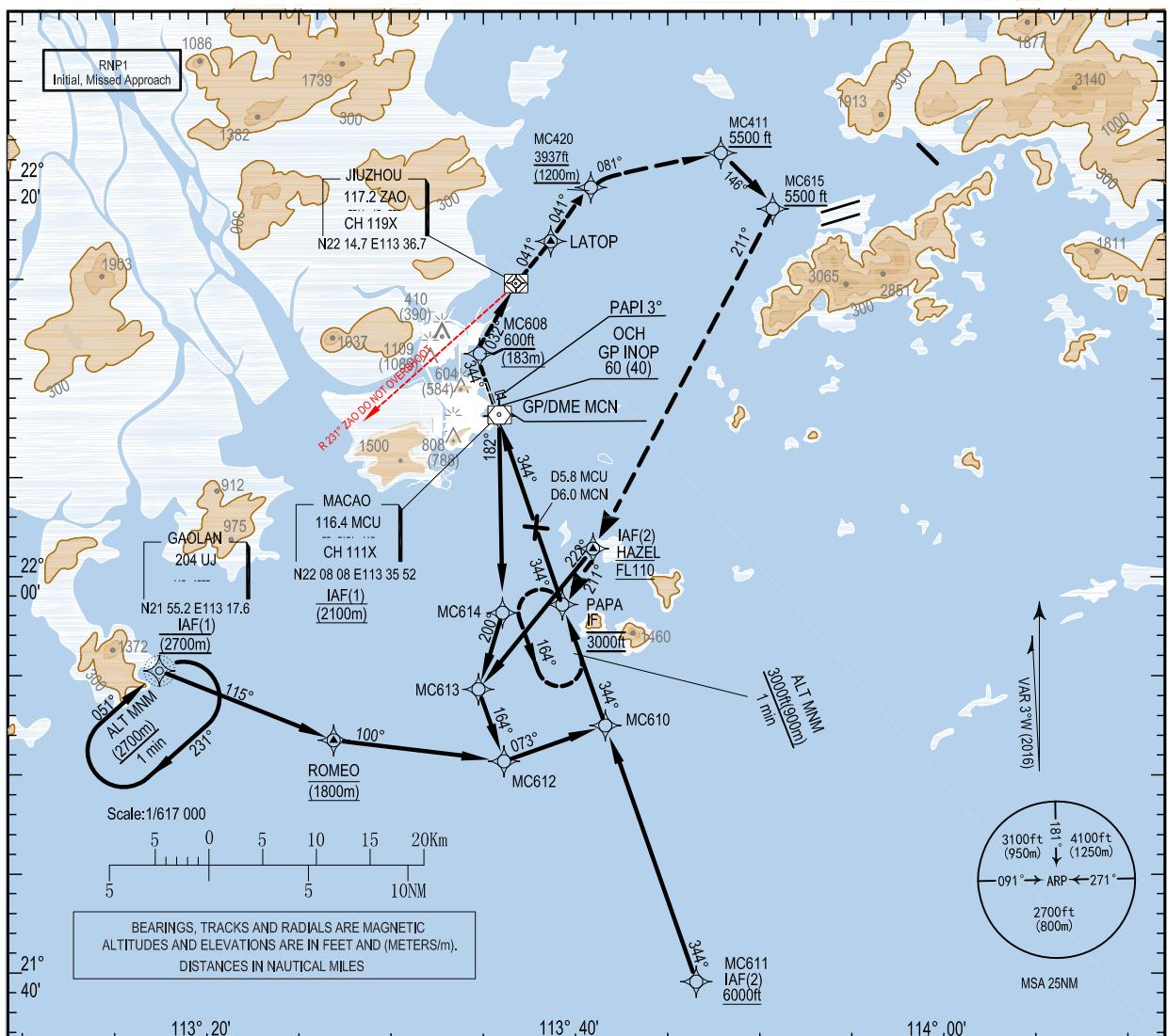
**MISSED APPROACH (2):** (MNW climb gradient 5.4% required until passing 5500 ft) Climb to MC608 at 600ft (183m) or above, turn right track to ZAO, LATOP, MC420 at or above 1200m (3937ft). Track to MC411 at or above 5500ft and continue climb to 6000ft or as instructed by ATC. Then fly by MC615 on track 211°M to HAZEL, PAPA. When requested, join the holding pattern at PAPA at 3000ft or above, or proceed as directed by ATC.
