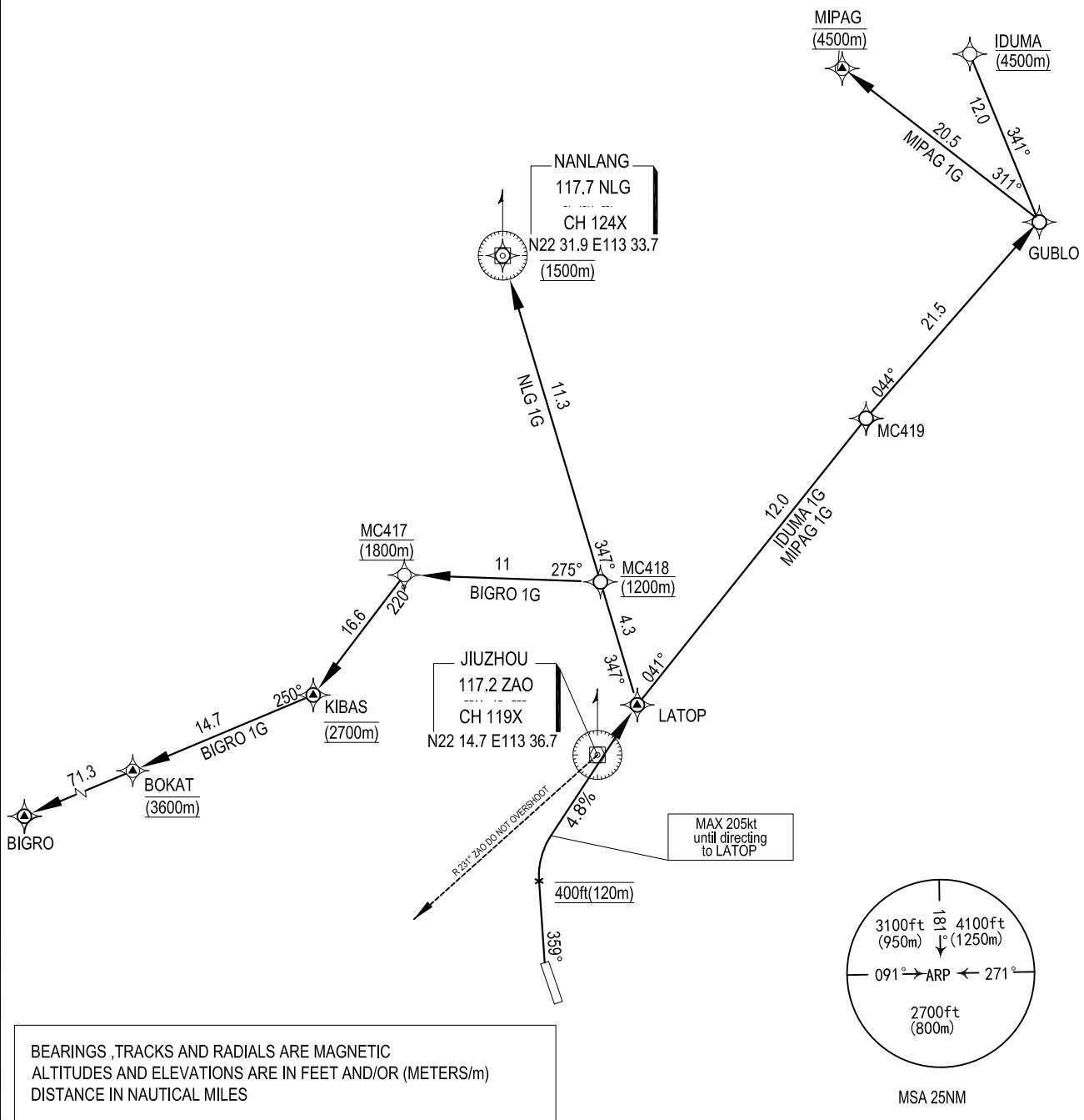
The procedure applied to BASIC RNP1, GNSS required.
