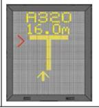
off as the aircraft approaches stop (reducing the length of the bar, bottom upwards) and as the last row turns off, less than the interval for one row remains until STOP appears.
