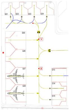
AIRCRAFT PUSHBACK / TOW PROCEDURE FOR BREAKAWAY POINT "Z" (RWY 34 / 16) Stands G13 – G15
